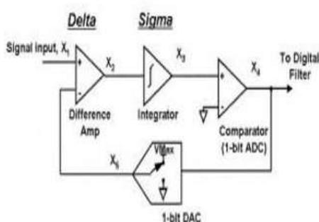
Fig 6.2 Delta-sigma ADC
